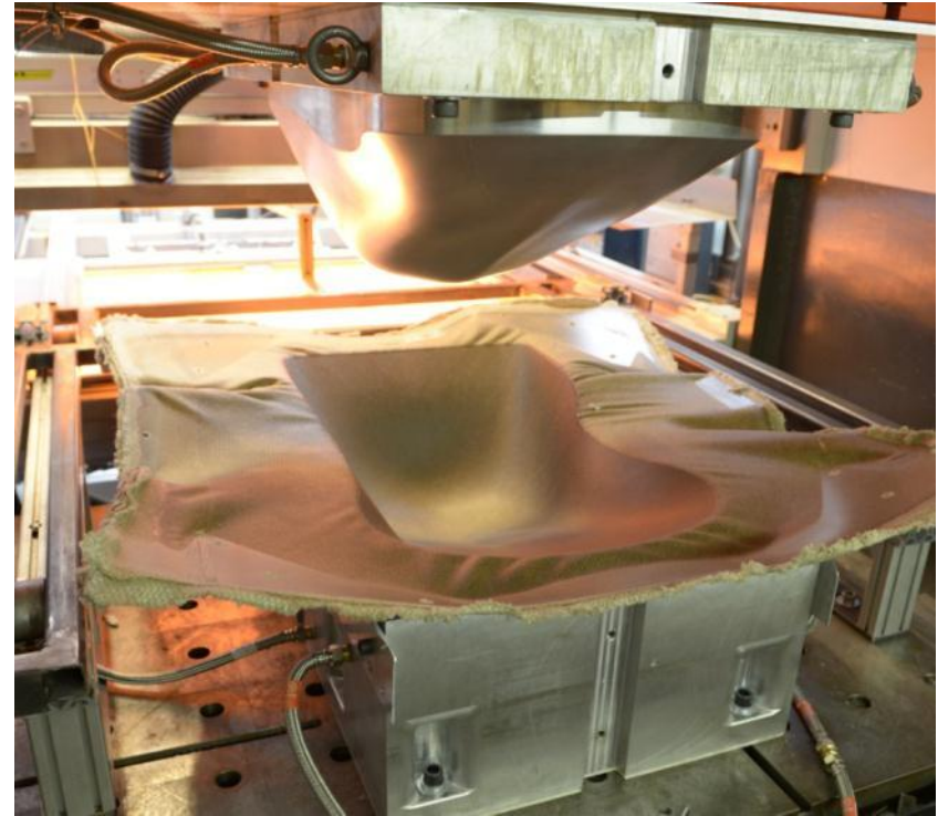
Production of car seat from biocomposites
