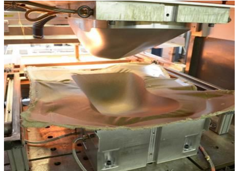
Car seat demonstrator develop from flax-PLA composites
